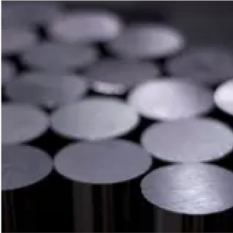
*Alloy 188 is known for its superior resistance to corrosion and oxidation at elevated temperatures, this is due to its composition, containing significant quantities of cobalt and chromium. This allows Alloy 188 to be well suited for high temperature environments. The alloy maintains structural integrity when exposed to extreme heat, oxidising agents, and corrosive media that would rapidly degrade many conventional materials.*
