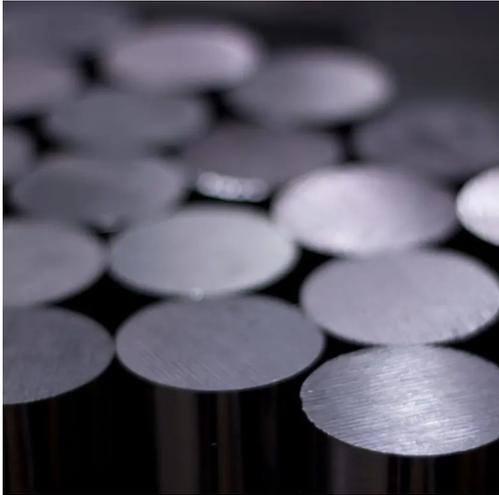
*Known as commercially pure nickel: Nickel 200 and the low carbon variant, Nickel 201, are utilised mostly for their excellent corrosion resistance.*
